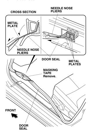
19. Remove the masking tape from the door seal.
