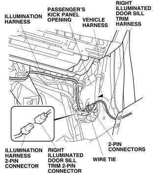
57. Secure the 2-pin connectors to the vehicle harness with one wire tie.
