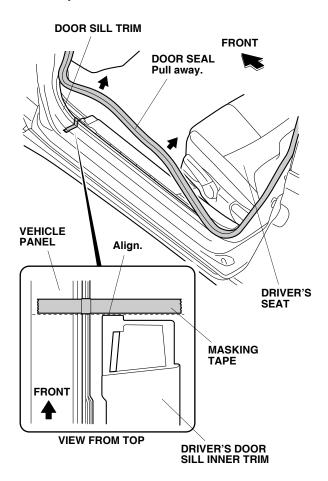
Attach a piece of masking tape to the vehicle panel.
